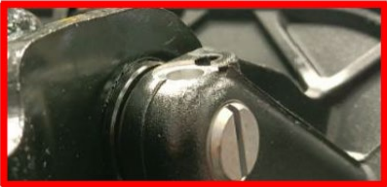
BAD PART – missing screw
