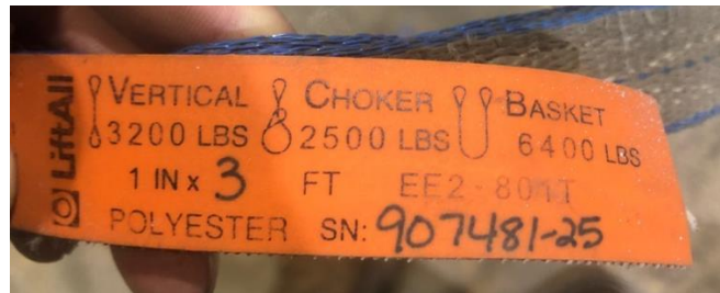
Figure 15: Rigging for lifting Upper ESS Enclosure
