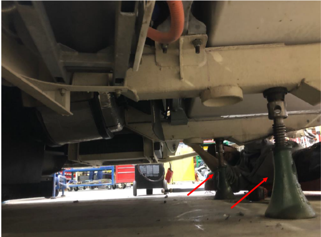
Figure 3: Support Rear Frame Members with Jack Stands
