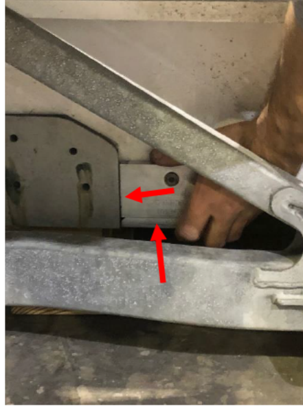
Figure 21: Place Fixture Against Corner Bracket as Shown
