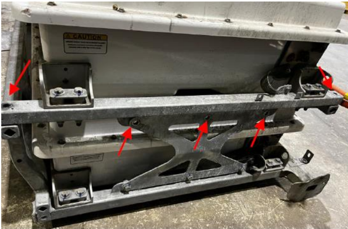
Figure 14: Remove Upper Cross-Brace Hardware (5 Places Each Side)
