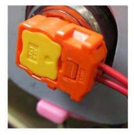
Once alignment is confirmed, push down firmly to engage the connector. When fully seated, press down on the yellow tab locking the connector to the inflator.
