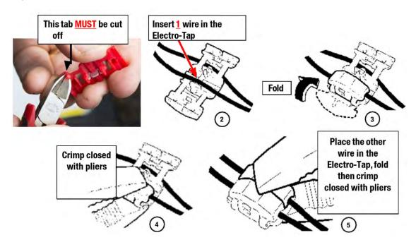
**STEP 4-** Once the Electro-Tap connector is fully crimped in place, cut the 2 wires on the **body harness connector side** of the Electro-Tap connector.
