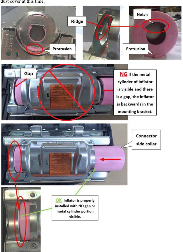
**STEP 9-** Install the new stopper plate over the harness connector end of the new inflator.
