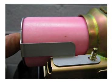
Always hold the stopper plate tight against the inflator as shown when installing and tightening the NEW self-locking nuts.
