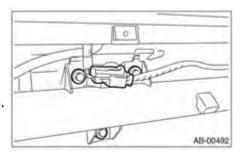
**STEP 2:** Visually inspect the airbag inflator positioning.
