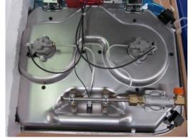
7. Visually inspect the gas tubes connecting the gas valve to the burner orifice holder for any cracks, splits, etc. Ensure no gas lines are loose by <u>gently</u> pulling the tubing along its axis away from each brass nut. <u>Use only two fingers.</u> If any gas lines are loose, stop the recall kit process and request a replacement unit by contacting Suburban Tech Support at 574-247-9235, option 5.
