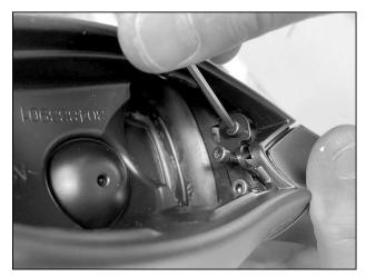
**NOTE:** To ease installation, use a 3mm round head insert.
