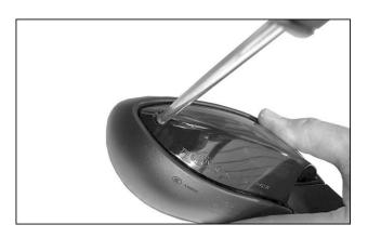
2. Gently lift the mirror cap using a small Allen Key, then push the cap out of location as shown on picture to remove it from assembly. Discard the cap.
