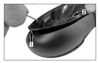
3. Using a 3mm Allen Key, remove and discard the three (3) socket head screws and metal plate.
