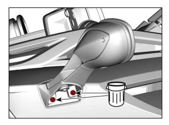
2. Gently pull the mirror housing and disconnect the mirror light harness connector.
