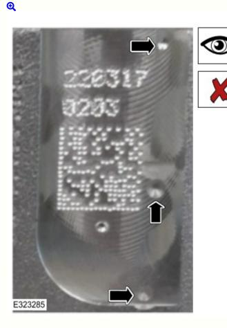
7. The failure condition shown highlights 2 drilled tooling marks in the upper and middle right side of the tooling stamp.
