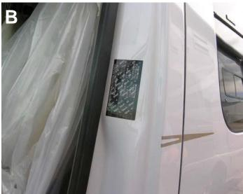
2. Clean the OEM label face with isopropyl alcohol and cover the OEM Tire Inflation Pressure Label with the new Tire and Loading Information Label (Label 1). See Photo C
