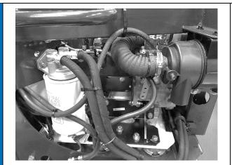
Secure oil and fuel lines with with cable ties to prevent them from being rubbed, pinched, or damaged.
