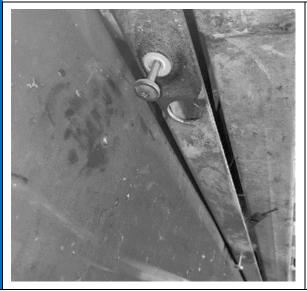
Install the five Torx bolts with a nylon washer halfway in each of the holes at the rear of the unit.
