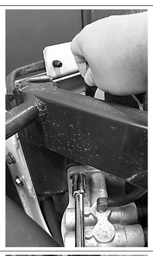
Remove hardware securing oil and fuel filter base to the frame.
