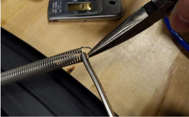
Figure 11a: Hold the ER bar and pull the spring hook with the pliers.
