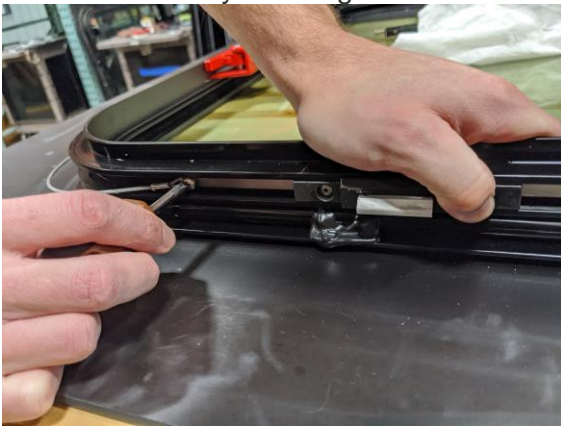
Figure 27a: Installation of ER bar screw.
