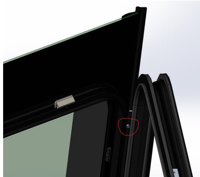
Figure 2b: Hinge retention screw circled in red.
