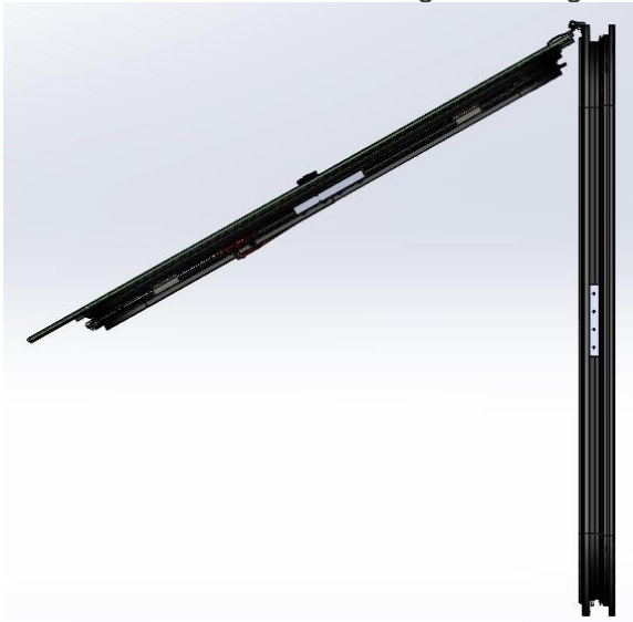
Figure 2a: Mainframe open to expose hinge retention screws.
