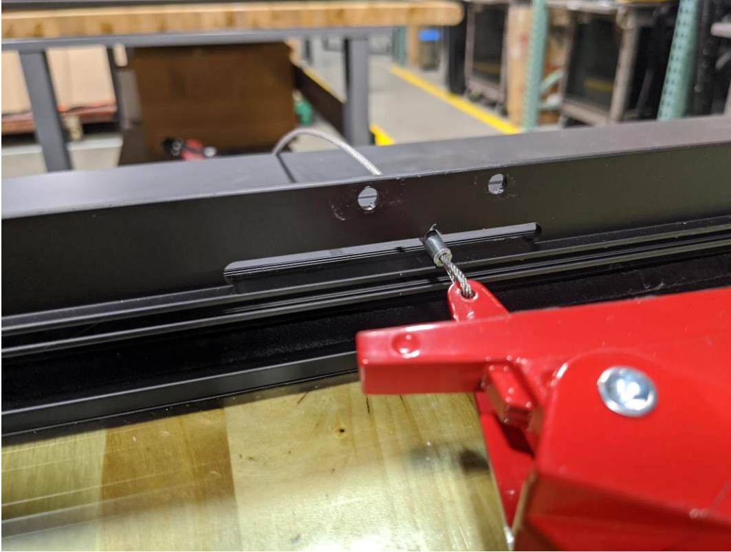
Figure 13: Use enlarged section of slot cutout to slide cable loops through.
