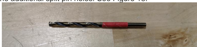
Figure 18: Drill bit taped for depth indication.
