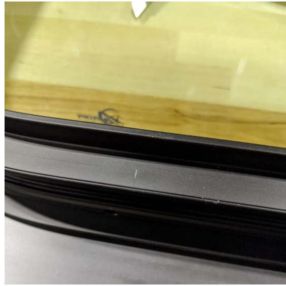
Figure 16b: Scored mark on the frame.
