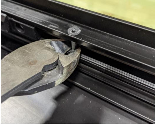
Figure 6a: Pliers gripping split pin.
