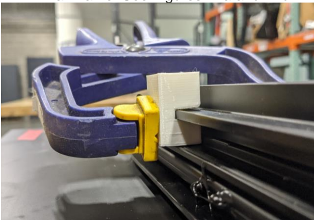
Figure 17a: Drill jig clamped correctly.
