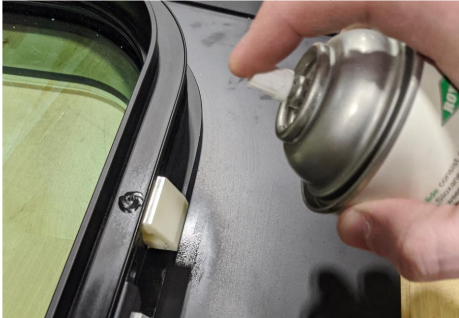
Figure 35: Silicone spray lubricant applied to locator block.
