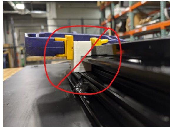
Figure 17b: Drill jig clamped incorrectly.
