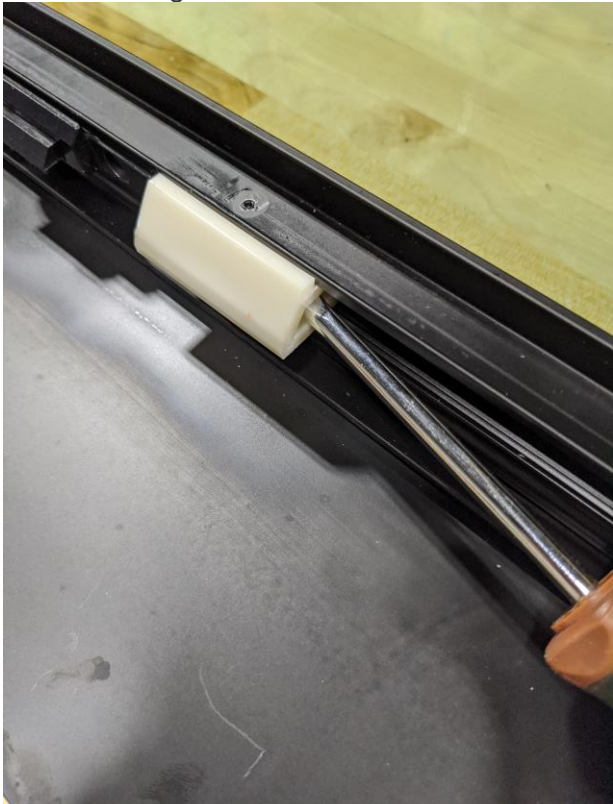
Figure 5a: Flat head screwdriver wedged in the side of the locator block.
