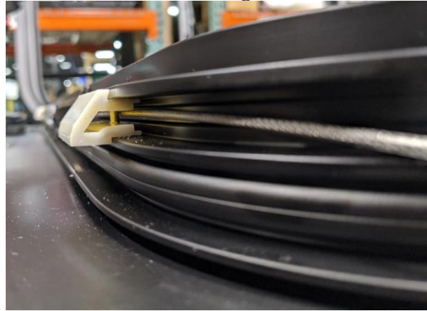
Figure 23b: ER cable fed under locator block.
