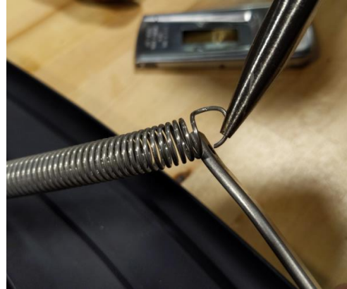
Figure 11b: Pull the hook open with the pliers and slide the ER bar out.
