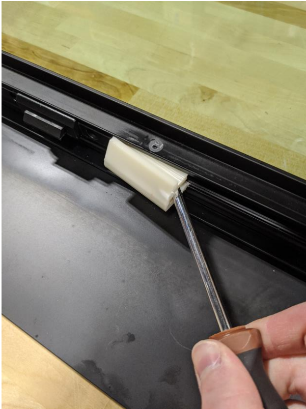
Figure 5b: Locator block pried out of ER track.
