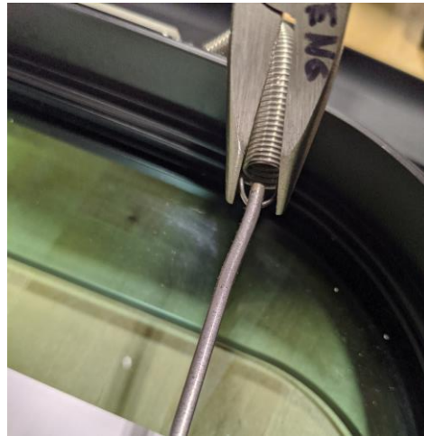
Figure 24b: Bend spring hook closed.
