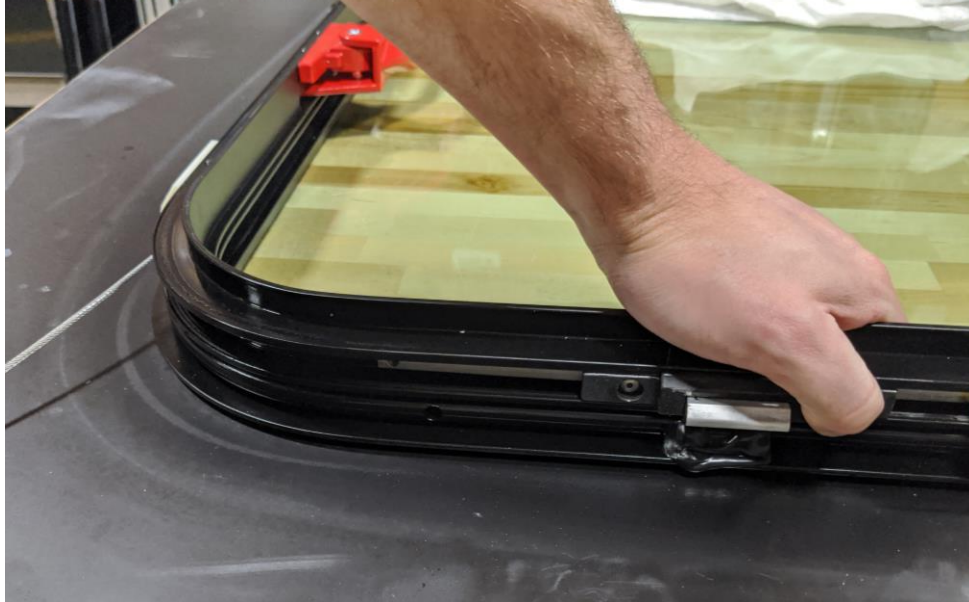
Figure 26: ER bar held in place with enough room to install ER handle cable.
