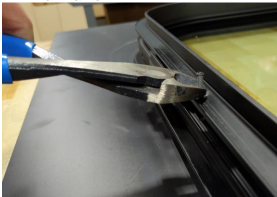
Figure 8a: Split pin gripped from interior of frame.
