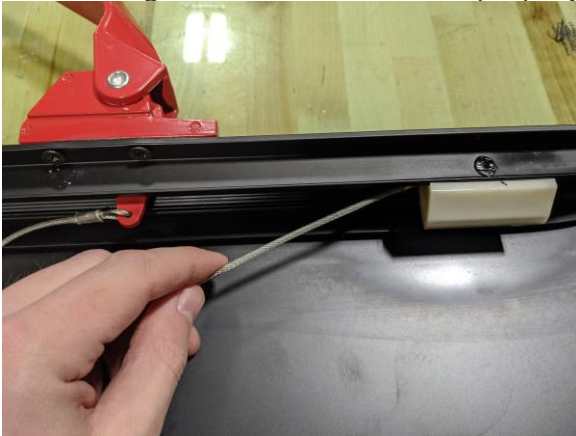
Figure 23a: Feed ER cable under locator block.
