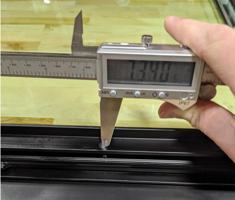
Figure 15a: Jaw hooked on original split pin hole.
