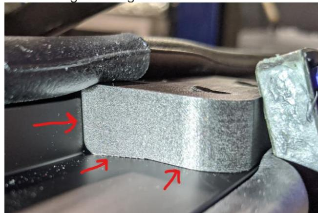
Figure 33b: Drill jig properly seated on the indicated edges.
