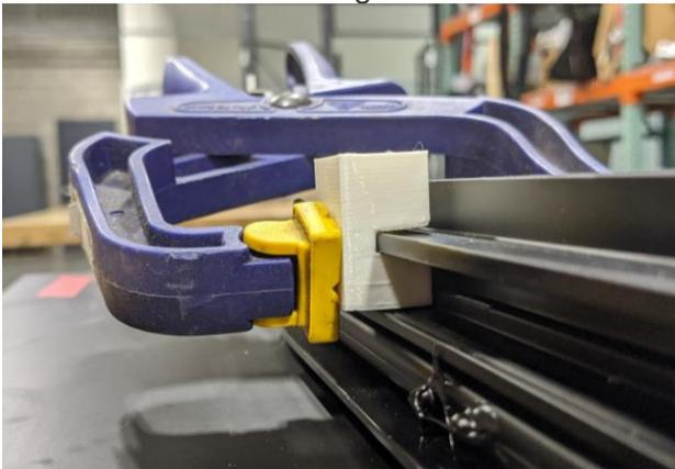
Figure 15a: Drill jig clamped correctly.
