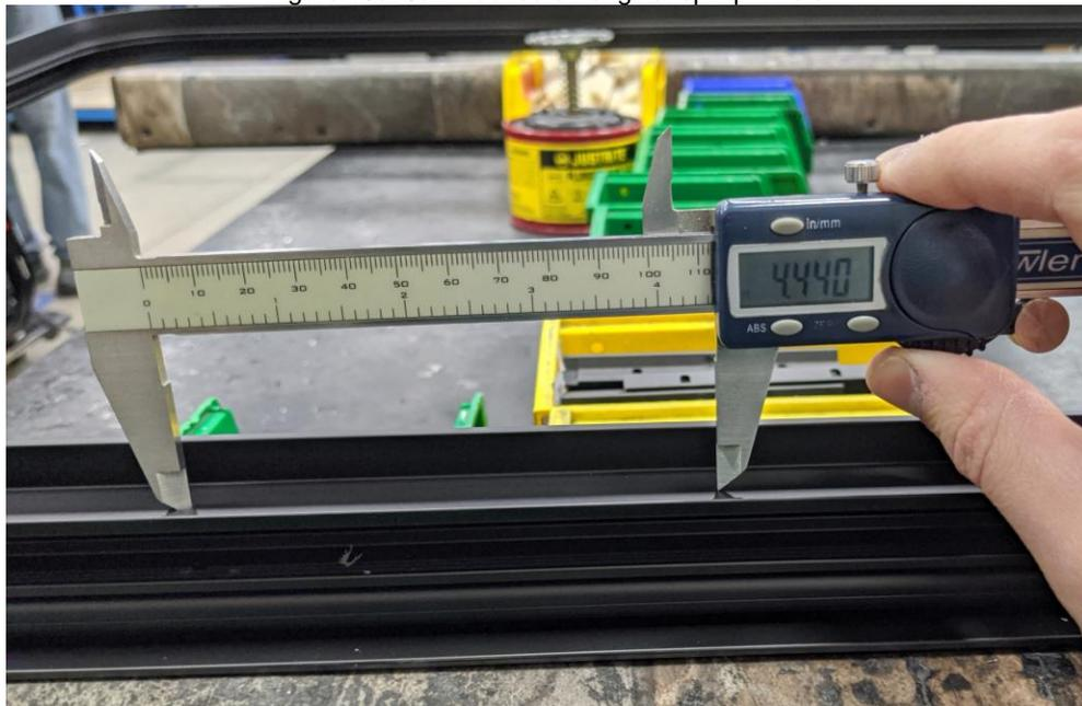
Figure 13b: Caliper extended to dimension for additional split pin.
