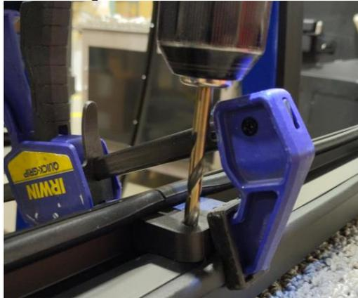
Figure 34: Drill aligned in drill jig.
