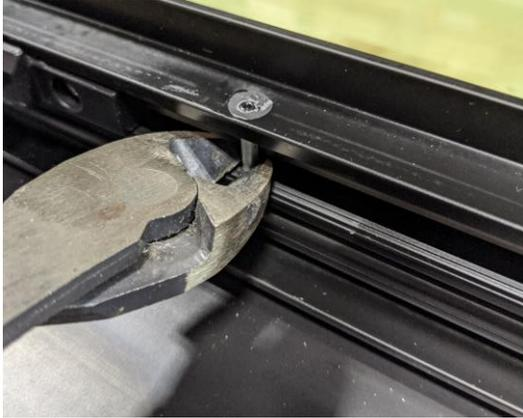
Figure 6a: Pliers gripping split pin.
