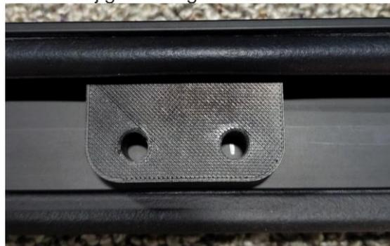
Figure 32: Right-side hole of drill jig aligned to mark on subframe.
