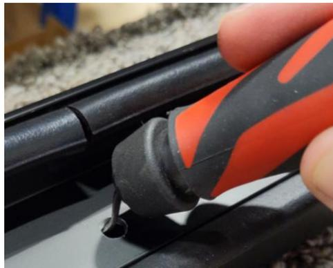
Figure 35: Deburr holes after drilling.
