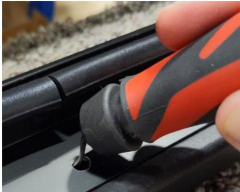
Figure 35: Deburr holes after drilling.
