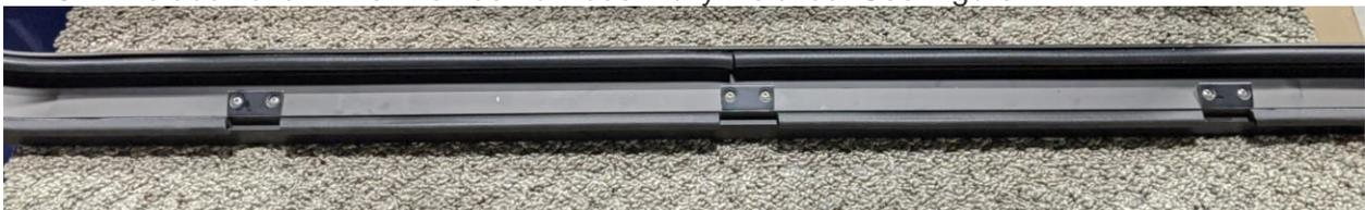
Figure 41: Subframe sill with additional strike fully installed.
