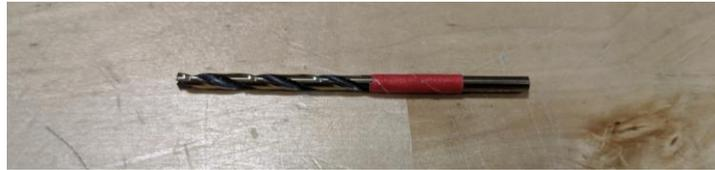
Figure 16: Drill bit taped for depth indication.
