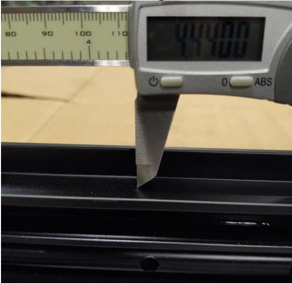
Figure 14a: Jaw used to score frame.
