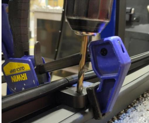
Figure 34: Drill aligned in drill jig.
