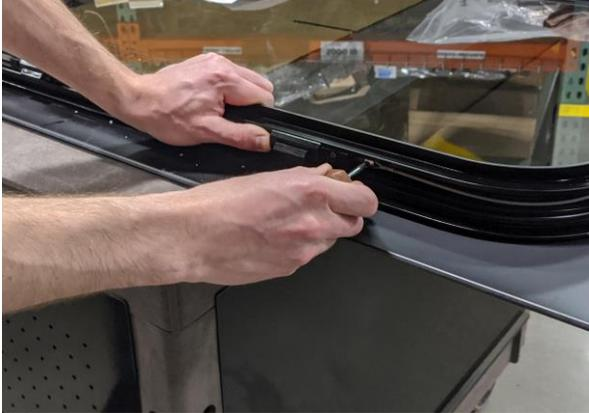
Figure 21a: Installation of ER bar screw.
