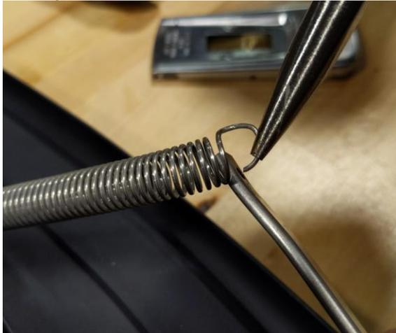
Figure 18a: Install spring hook into jogged end as shown.
