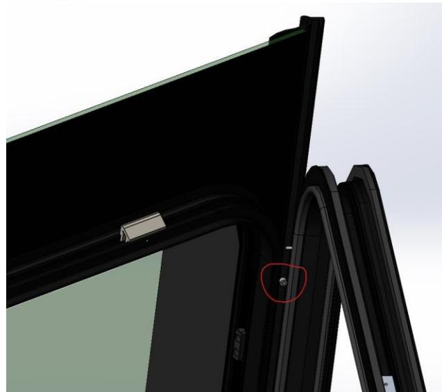
Figure 2b: Hinge retention screw circled in red.
