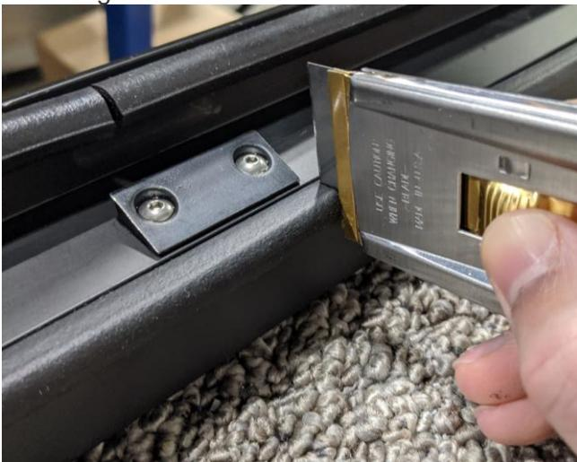
Figure 40a: Blade scraper cutting seal.
