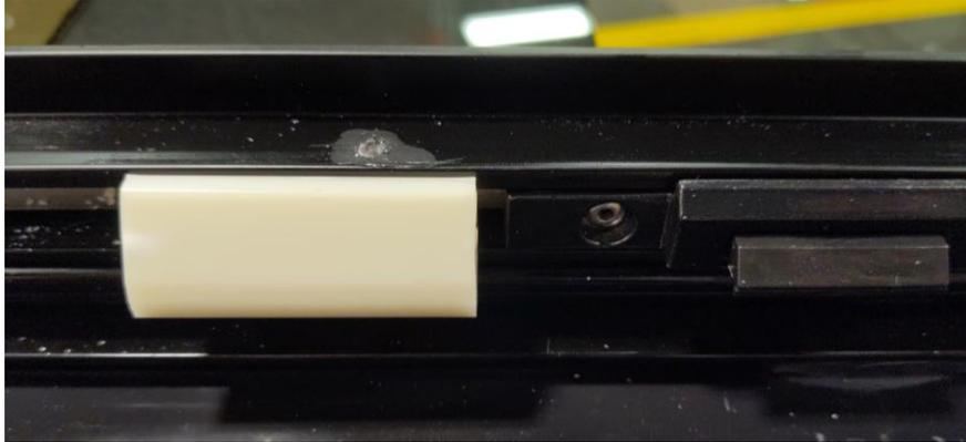
Figure 24: Offset locator block with gap between ER latch and block.
