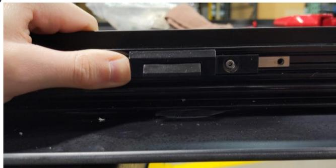
Figure 20: ER bar held in place with enough room to install ER handle cable.
