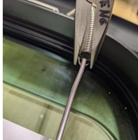
Figure 18b: Bend spring hook closed.
