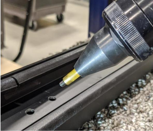
Figure 36a: Rivet nut installation tool.
