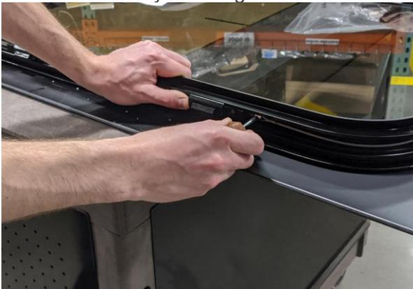
Figure 21a: Installation of ER bar screw.
