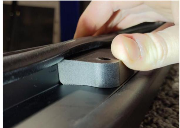
Figure 31b: Drill jig sitting on subframe sill.
