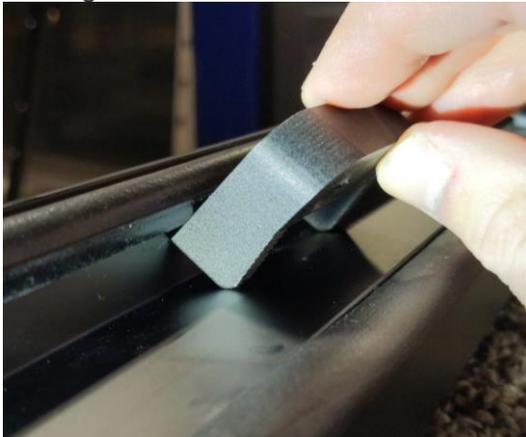
Figure 31a: Drill jig tipped under inner subframe seal.
