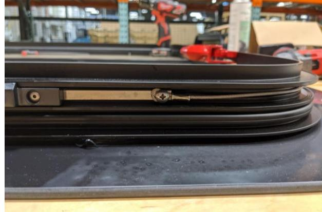
Figure 21b: Screw partially installed with ER cable loose.
