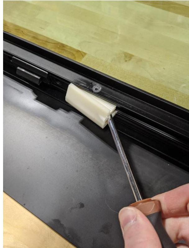
Figure 5b: Locator block pried out of ER track.
