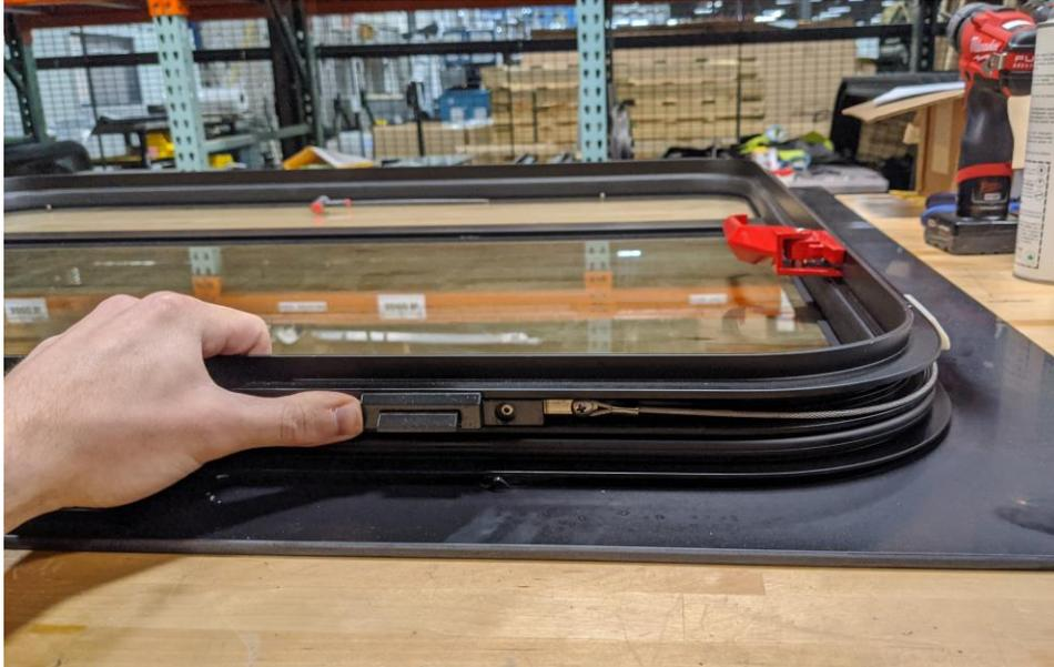
Figure 9: ER bar slid towards ER handle creating slack in ER cable.
