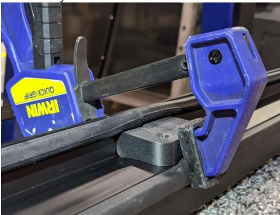
Figure 33a: Drill jig clamped in place.
