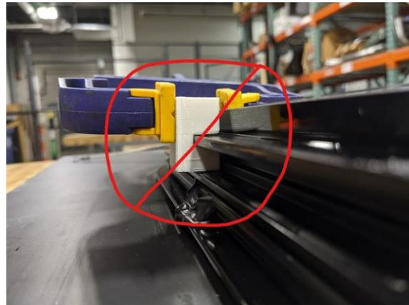
Figure 15b: Drill jig clamped incorrectly.
