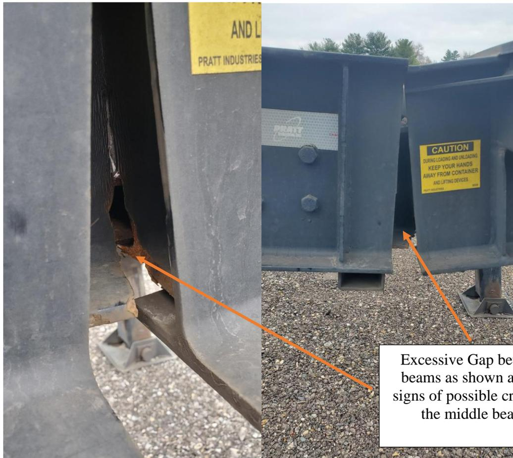
Excessive Gap between beams as shown are the signs of possible cracks in the middle beam.
