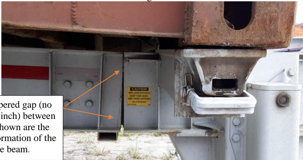
Minimal tapered gap (no more than 1 inch) between beams as shown are the signs of deformation of the middle beam.
