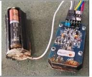
3. Cut the gray and white wires to release the battery pack from the remote.
