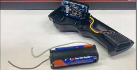
5. With battery pack removed, replace the remote control cover and the three screws.
