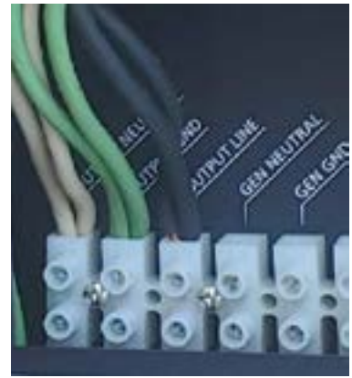
Figure 8 — 120-Volt Double Connection AC Output Wiring
