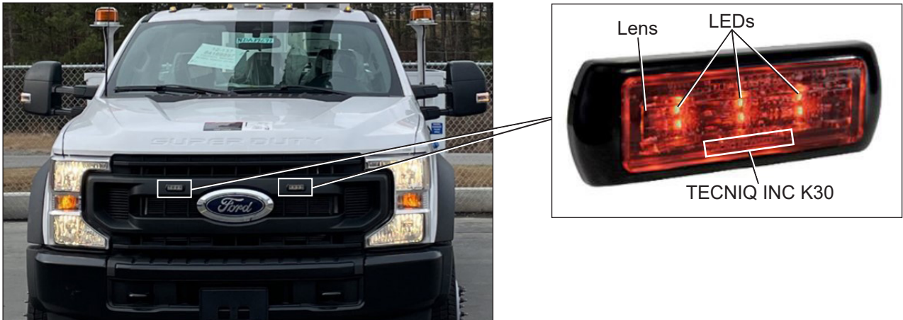
Figure 1 — Inspecting Surface-Mount Strobe Lights
