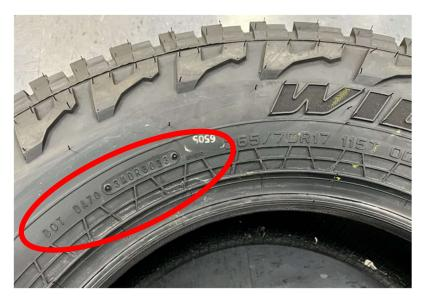
The mold number is located after the TIN as shown circled in red below.
