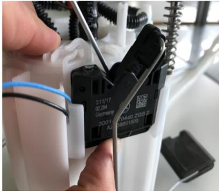
Figure 7 (using a screwdriver, carefully push float-and-lever sensor housing away from module housing and at the same time push float-and-lever sensor housing upwards.)
