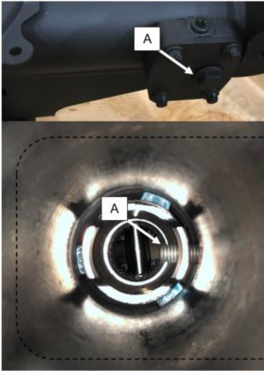
Figure 31 (delivery condition of bolt)
