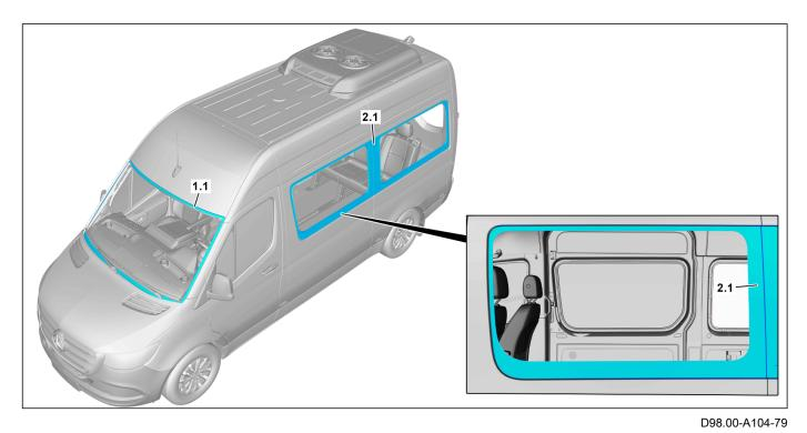
1.1 Windshield contact surface 2.1 Side window contact surface
