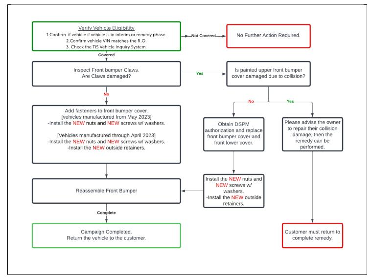
Note: If the painted upper front bumper cover is damaged from obvious collision, please advise the owner to repair their collision damage, then the remedy can be performed.
