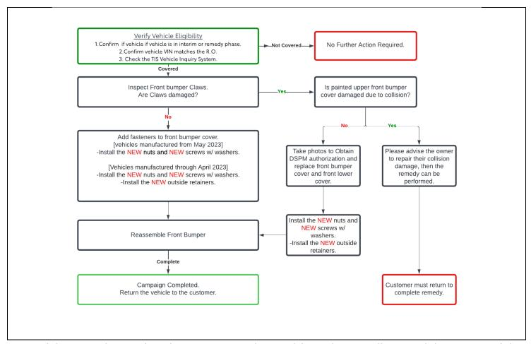
Note: If the painted upper front bumper cover is damaged from obvious collision and the integrity of the bumper is compromised, please advise the owner to repair their collision damage, then the remedy can be performed. If the painted bumper portion damage is cosmetic and the mounting claws are not damaged it is ok to perform remedy.
