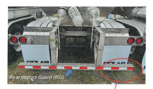
1) Tag will be installed on the passenger side of the RIG, on the forward side.
