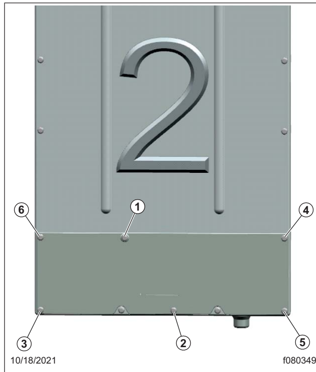
Fig. 10, Inverter Access Cover Tightening Sequence
