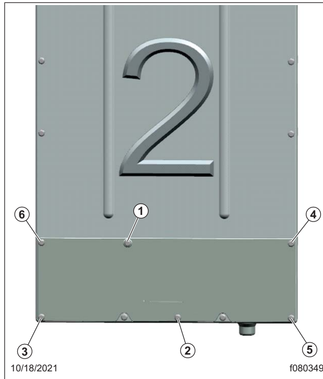
Fig. 10, Inverter Access Cover Tightening Sequence
