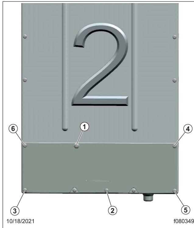
Fig. 10, Inverter Access Cover Tightening Sequence
