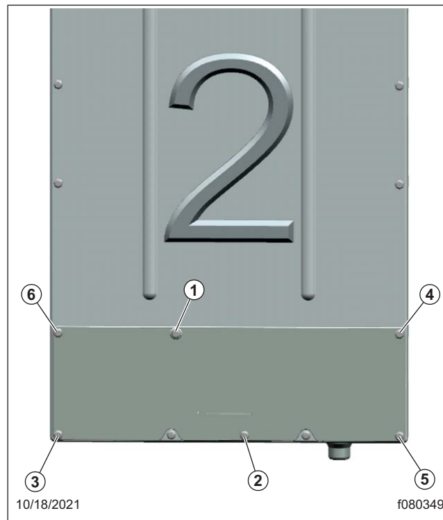
Fig. 10, Inverter Access Cover Tightening Sequence
