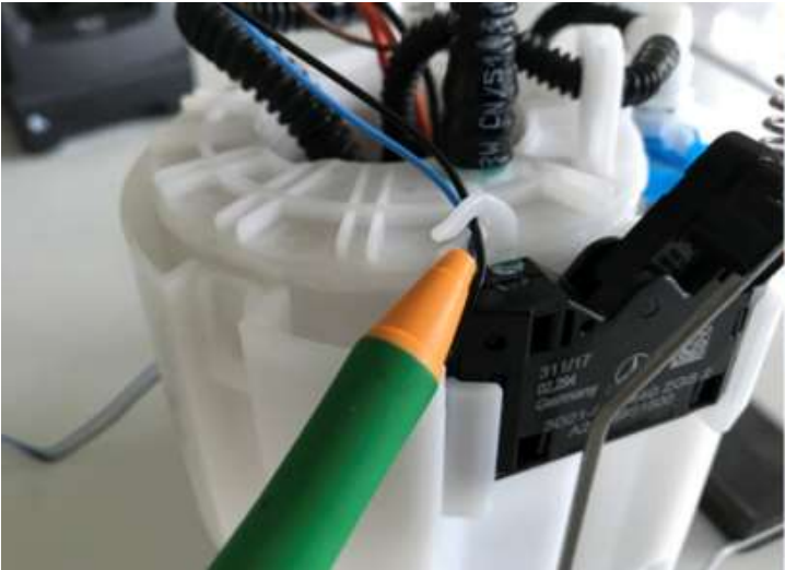
Figure 4 (remove lines from routing clip)
