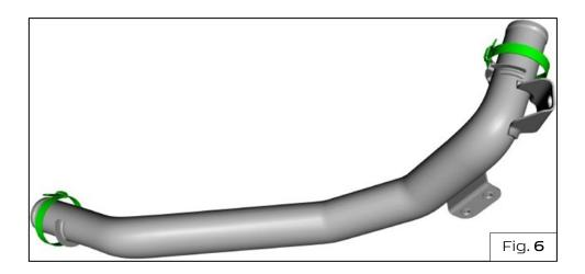
> Place the connecting pipe on the vehicle and insert the two ends into the respective hoses - Fig. 7.
