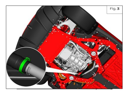
> Pull out and remove the fuel tank connecting pipe from the relative hoses - Fig. 4.
