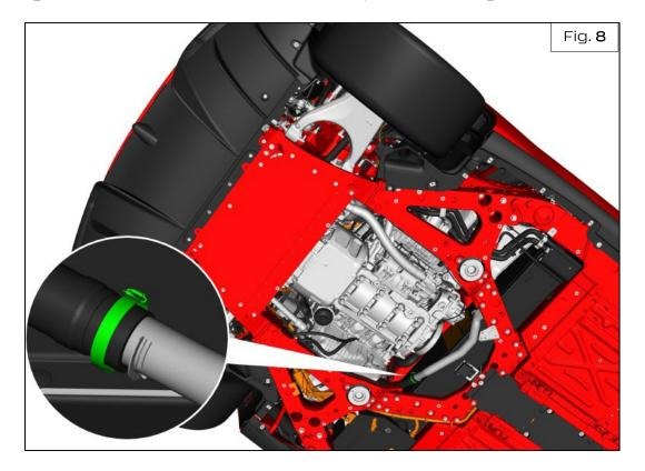
> Tighten the indicated screw collar to a torque of 4 Nm - Fig. 9.
