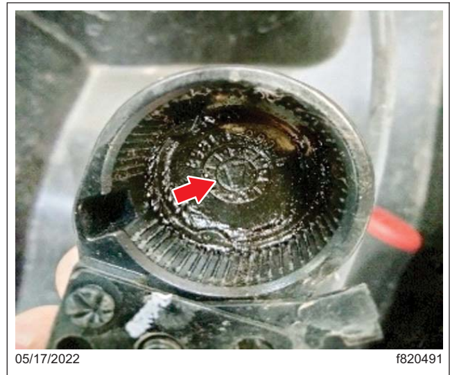
Fig. 2, Date Stamping on the Wiper Arm
