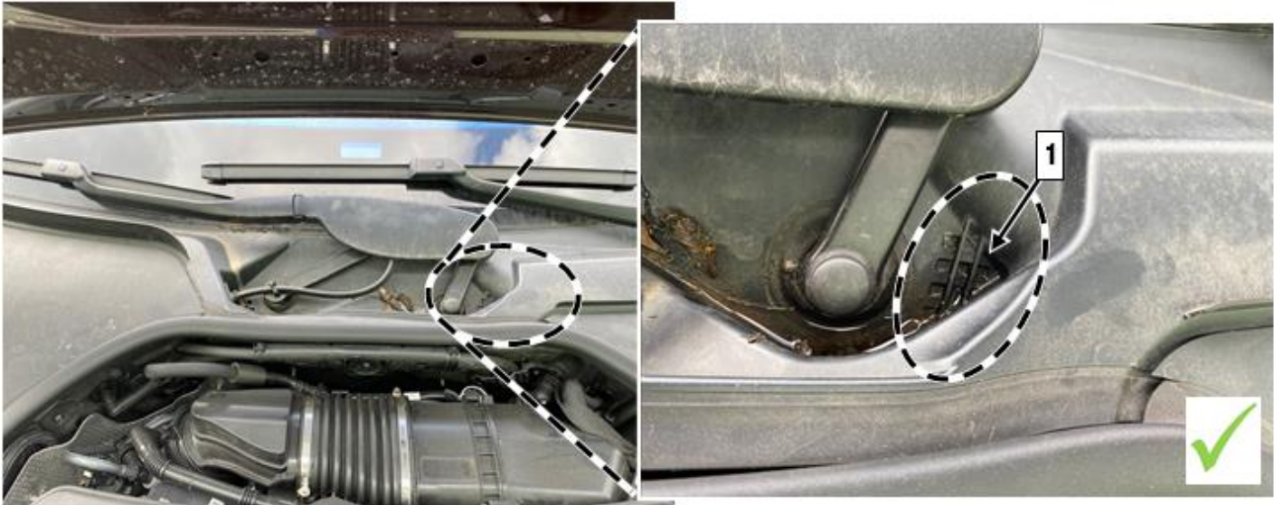
Figure 2 Drain of air/water duct OK
