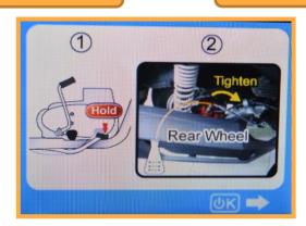
Hold the brake Pedal in pressed condition and tighten the bleeding nipple
