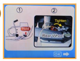
Hold the brake lever in pressed condition and tighten the bleeding nipple
