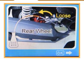
Loosen the bleeder nipple – (Brake lever in released condition ) 21
