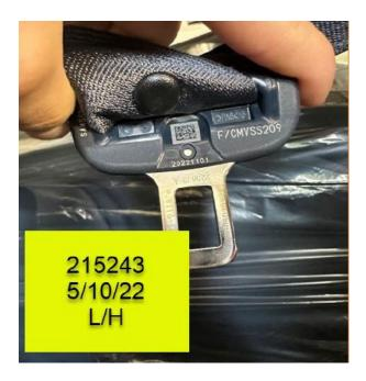
Acceptable STUI Photo of the Seat Belt Buckle Assembly with side noted, last 6 digits of VIN & date of repair (inspection passed, for GV60 vehicles ONLY)
