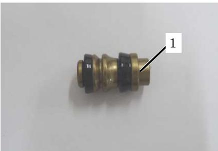
11) Install the new snap ring (1) using the special tool.
