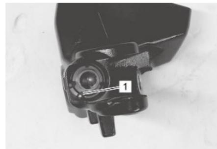
6) Remove the piston/cup set (1), return spring (2) and return spring guide (3) from the master cylinder body.
