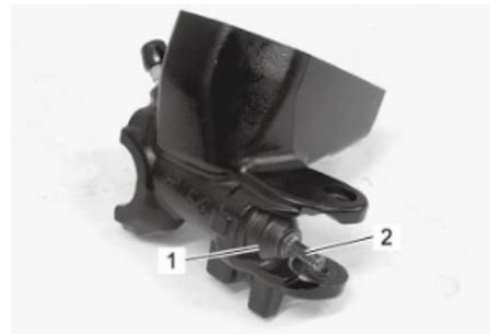
5) Remove the snap ring (1) using the special tool.
