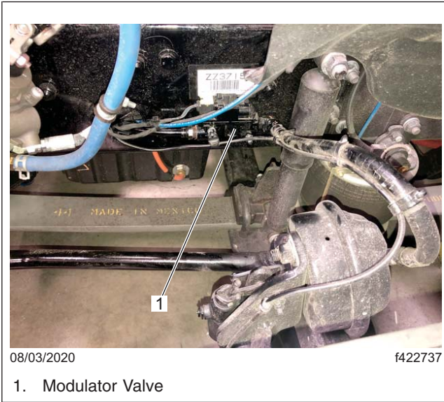
Fig. 2, Location of the Modulator Valve
