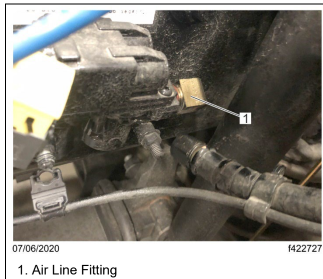
Fig. 9, Loosening the Brake Chamber Air Line Fitting
