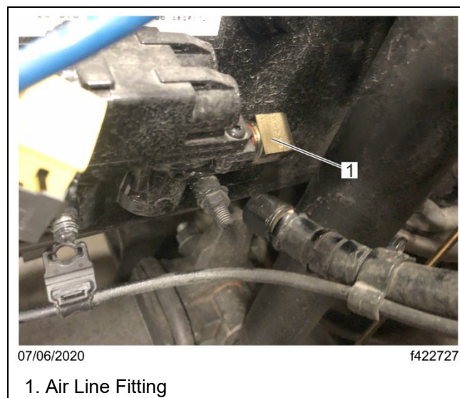
Fig. 9, Loosening the Brake Chamber Air Line Fitting
