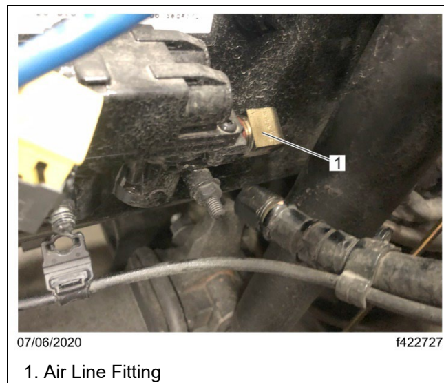
Fig. 9, Loosening the Brake Chamber Air Line Fitting
