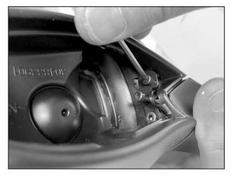
**NOTE:** To ease installation, use a 3mm round head insert.
