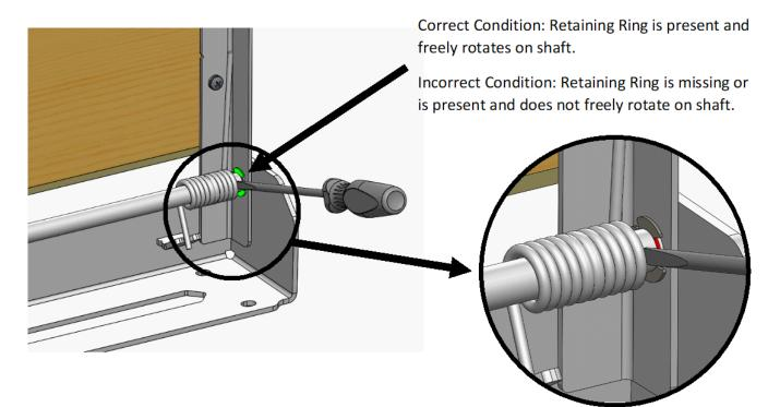
To verify if the Retaining Ring rotates freely on the shaft, the pressure from the spring on the Retaining Ring has to be relieved. Wedging a flat-headed screwdriver between the spring and the side of the seat is a good way to go about this. With one hand relieving spring pressure, try to rotate the Retaining Ring with the other hand.
