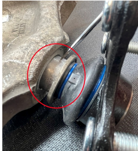
Steel insert has moved
