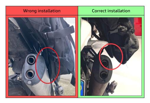
The defect analysis revealed that the assembly of this accessory as per instructions is not robust enough to avoid this risk if the customer does not take precautions when installing and using the KIT.
