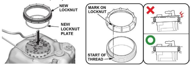
37. Tighten the fuel tank unit locknut to the specified torque.
