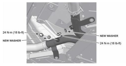
Disconnect the water hoses from the center pipes, and cap off the ends. Replace the water outlet hose during installation.
