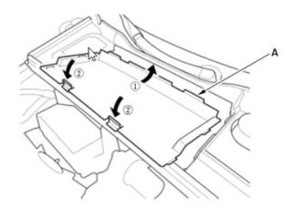
NOTE: Make sure that the 12-volt battery access cover is installed correctly and fully seated. Failure to do so will affect A/C performance.
