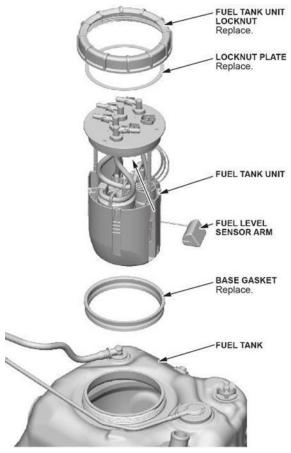
35. Partially insert the new fuel tank unit into the fuel tank with a new base gasket.
