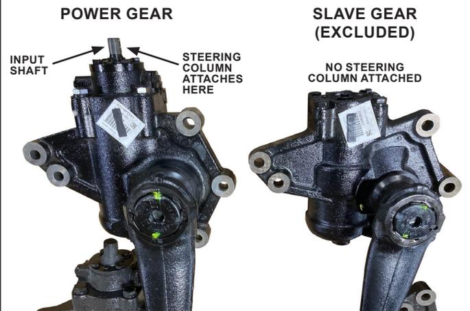
Figure 7 – Slave Gear Part Number and Image Example
