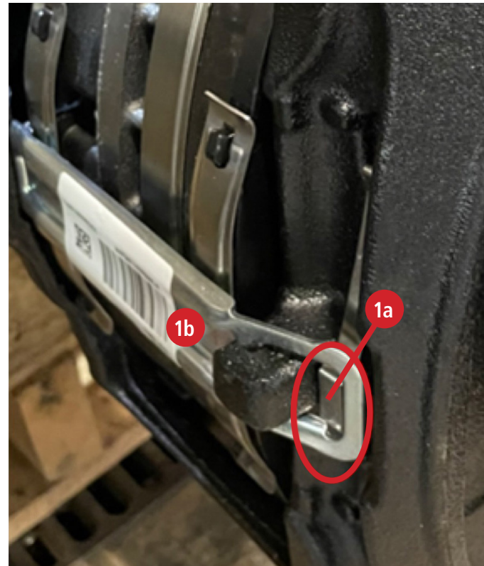
Spring bracket trapped under pad retainer
