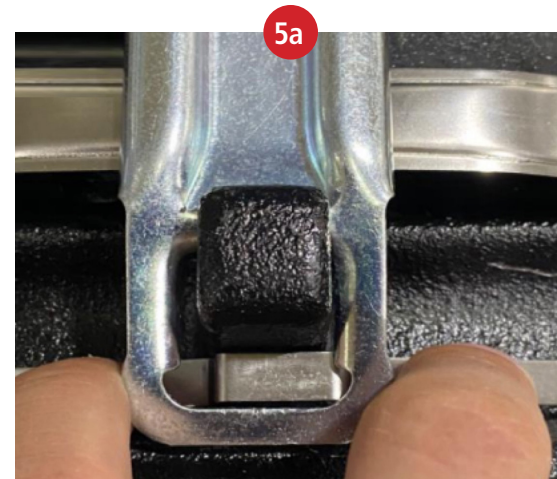
Top of spring bracket is trapped beneath edge of pad retainer bar.
