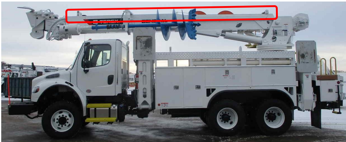
Figure 2. General Digger Derrick: Weld to Inspect – Main Boom
