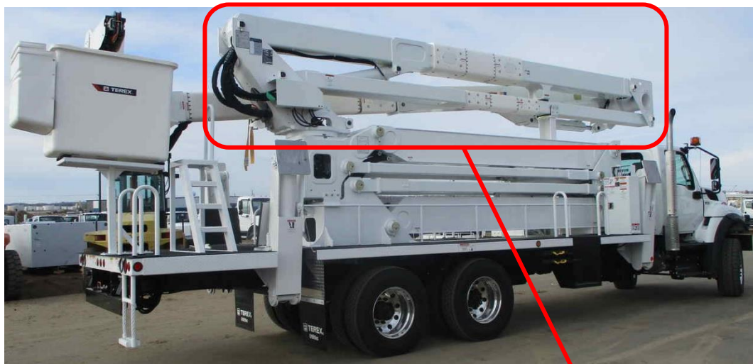
Figure 4. General Digger Derrick: Weld to Inspect – 2 nd , 3 rd , and 4 th Booms
