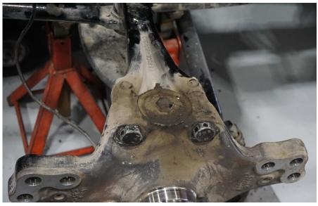
**Step 12:** Clean spindle for reinstallation.
