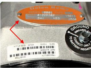
REMY 55S Alternator will have a Delco-Remy identification plate riveted to the body as well as a bar code sticker next to the ground stud as shown.
