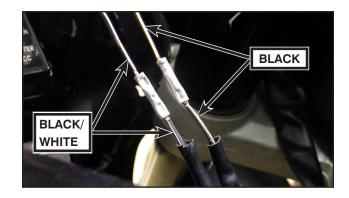
Crimp [C] both butt connectors firmly.
