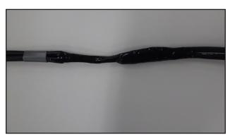
Route the harness [H] as shown so the clamp [C] is in the center of the repair.
