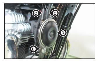
Cut each lead wire 80mm from the end of the lead connector.
