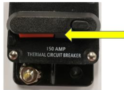
Figure 2: Bad Circuit Breaker with RED arm
