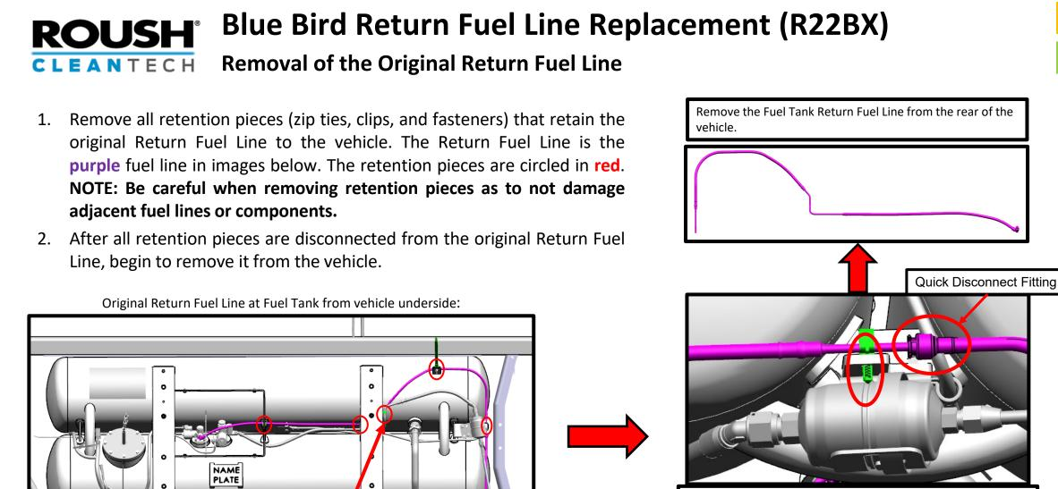
Disconnect the original Return Fuel Line at front of Fuel Tank. Press plastic tab on the quick disconnect fitting and pull the fuel line sections apart from each other. It may be necessary to snip the Fuel Line to the right of Quick Disconnect fitting if line separation is not possible due to corrosion. **DO NOT USE ANY CUTTING TOOLS THAT EMIT SPARKS**
