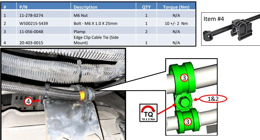
2. Secure both the existing Supply Fuel Line and new Return Fuel line with two Plamps adjacent to each other at the transmission mounting point. Use an edge clip cable tie on the left side of the bracket to secure the new return fuel line. A red tag on the new return fuel line will indicate the proper location to clamp the new fuel line in place with the Plamp.
