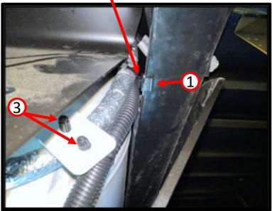
Ensure that the convoluted Return Fuel Line and original Supply Fuel Line are routed up towards the frame rail as shown. Use two fir tree cable ties (Item #1) to secure the supply and return fuel lines to the indicated retention tab. Then secure both the Supply and Return Fuel Line to the frame edge as shown using Item #1.
