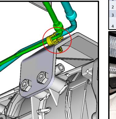
On top of the transmission, remove the snail clip (yellow) from the pictured bracket and discard.
