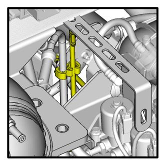
Behind the engine, remove Snail Clip and original Return Fuel Line tube (yellow).
