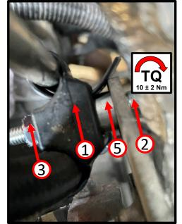
2. Install Dual Clamp Zip Tie and secure the new Return Fuel Line together with the Supply Fuel Line. Ensure that the 6mm Aluminum spacer is installed as pictured. NOTE: A red tag on the new Return Fuel Line will indicate the proper location to clamp the new fuel line in place.
