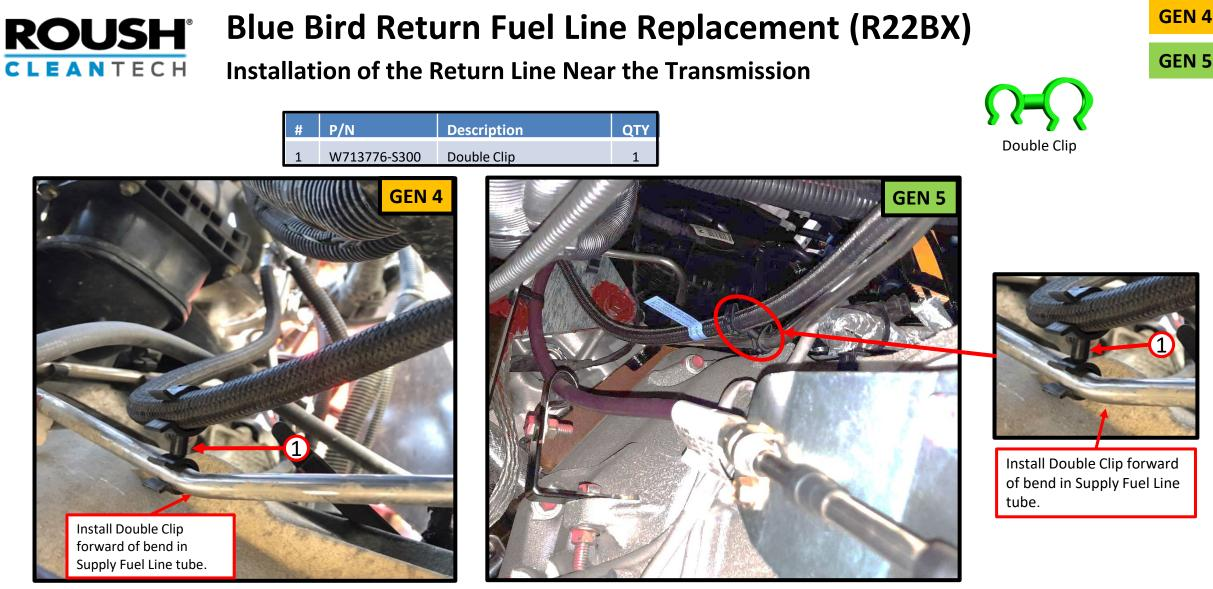
Near the top of the transmission, secure the flex hose (of new Return Fuel Line) to Supply Fuel Line with Double Clip. **NOTE: install the Double Clip immediately forward of the bend in the Supply Fuel Line Tube**
