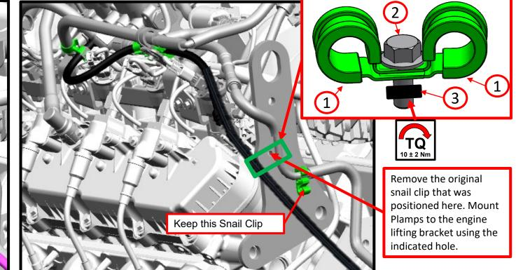
Just behind the engine, remove the existing snail clip and use two Plamps to retain the existing Supply Fuel Line and the new Return Fuel Line. A red tag on the return fuel line will indicate the proper location to clamp the new fuel line in place.
