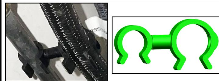
Use a Double Clip (Item #3) to maintain clearance between new Return Fuel Line and Supply Fuel Line tube.
